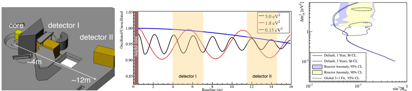
FIG. 1: Left: Engineering concept of ton-scale  $\bar{\nu}_e$  detectors at distances of 4-20 m from a reactor core. The NIST facility is shown as an example. Middle: Concept of probing short-baseline oscillation of unknown  $\Delta m^2$  with 2 or more radially extended detectors. Oscillations are detected either within one detector or between two detectors. Right: Sensitivity and discovery potential of a nominal short-baseline reactor experiment with 1 and 3 years of data. Figures from [10].
